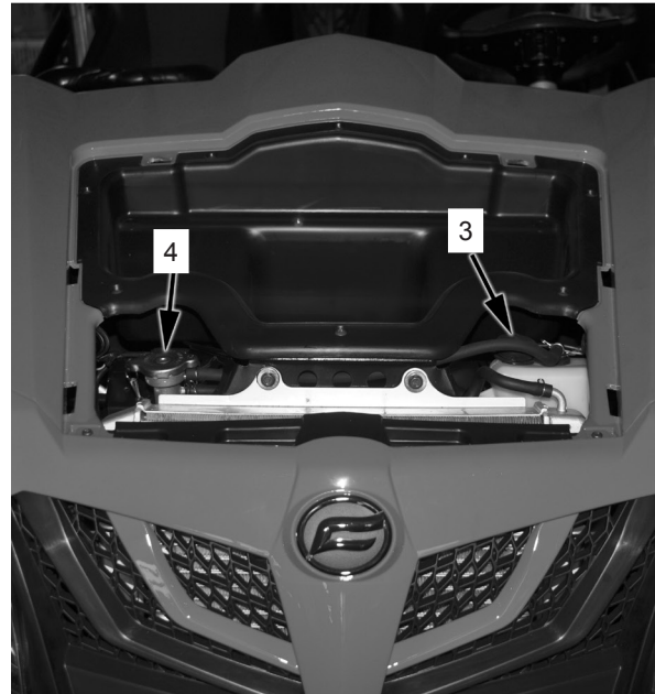
3. Reservoir Tank Cover
